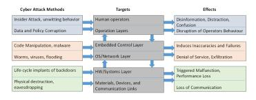
Fig. 1. Potential cyber-attack methods, targets and effects
