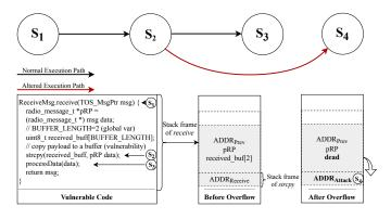
Fig. 2. Normal and Altered Control Flows
